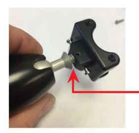
Clean off any Loctite residue from the threads of the ball stem, apply some Loctite 271 (Red) to the threaded hole in the clamp, screw clamp onto the ball stem and viola, you now have an old style Violin Bow Adapter!
