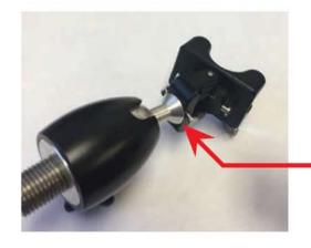
Use a hobby torch to heat the end of the ball stem where it connects to the yoke of the pivoting clamp assembly. This will help break the Loctite bond.
